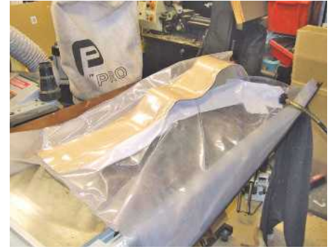
▲ Pic.12 These were made with several layers of veneers, each clamped tight to a former and put in a vacuum bag
